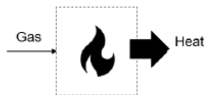
Figure 5. Representation of a stove and general water heaters that operate on natural gas.
